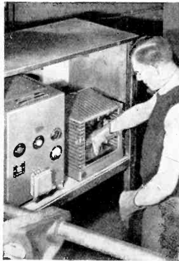
A comparatively simple case of effective anti-interference screening: the "work" chamber of a Rediffusion \frac{1}{4} kW heater, mounted close to the generator and fully screened.
