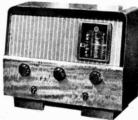
One of the things for which the author of this article pleads is an adequate short-wave tuning system—a rarity even in the best of pre-war broadcast receivers. Here is one of the exceptions; the Murphy A76, which gave many of the refinements of a "communication" receiver at moderate cost.
